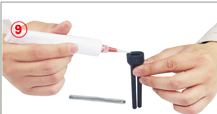
9: Pour RTV silicone inside the main hole of the two holes silicone boot.
