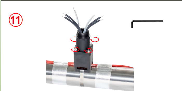
11: Compress the seal by screwing the upper part of the foot with the 4 screws until the both parts are in touch
