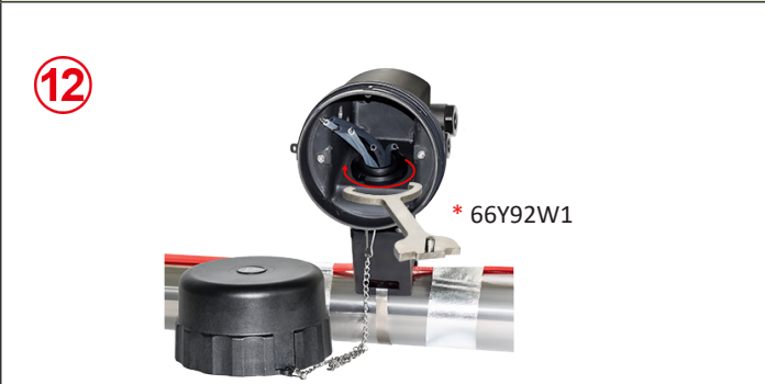
12: Place the gasket in the upper recess of the foot, then the box above. Orient the housing according to the desired position, then place and tighten the toothed nut until it locks.
